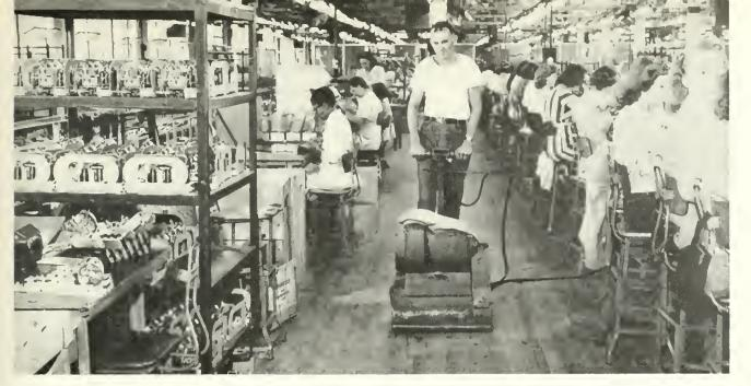
AMPLE AISLES, ADEQUATE LIGHTING AND FLOORS KEPT SPOTLESS BY SANDING MACHINES ARE TYPICAL FEATURES OF THE "HOUSEKEEPING" PROGRAM FOLLOWED AT REA'S BLOOMINGTON, INDIANA, PLANT.
