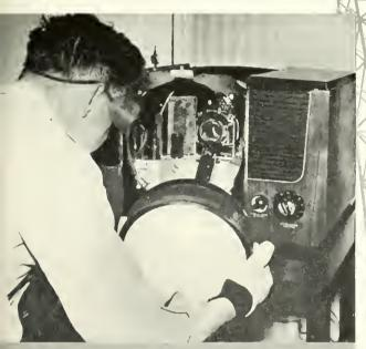
A 10-inch RCA kinescope is inserted into the socket of the television receiver to complete the installation inside the home.
